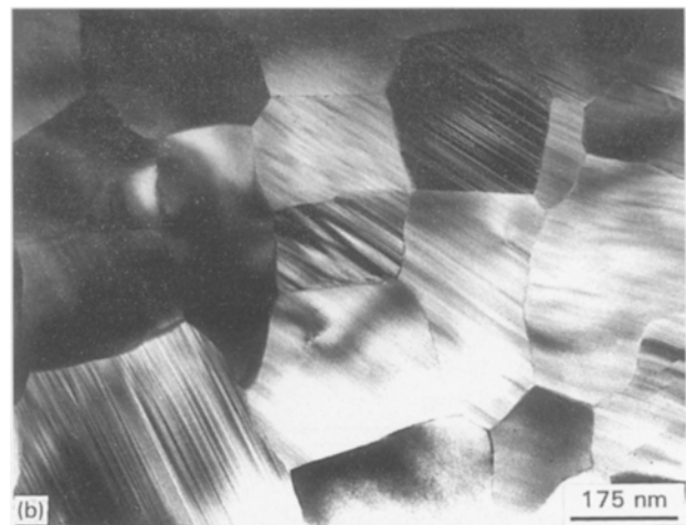
Figure 8 Plan view micrograph, showing (a) FeSi microstructure, of sample annealed at 650°C for 10 min, and (b) \beta -FeSi 2 sample annealed at 650°C for 1 h.
